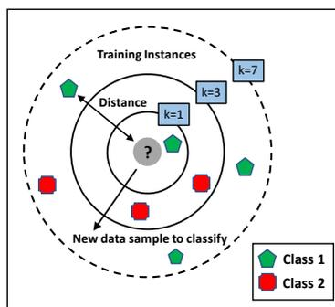
Fig. 2. A demonstration of KNN algorithm
