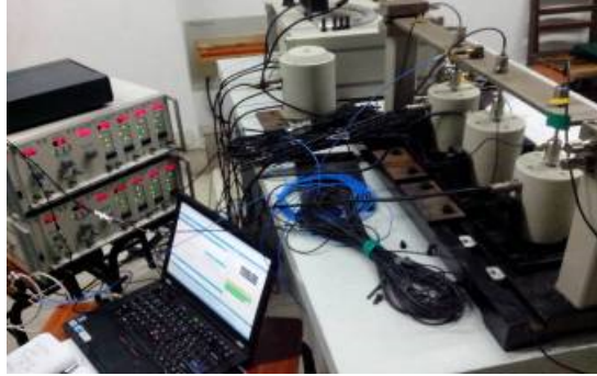
Fig. 8. Identification test of excitation sources of cantilever beam
