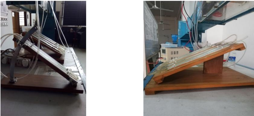
Fig. 3. Inclined manometer
