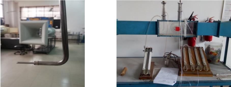
Fig. 1. Three tube probe yaw meter setup
