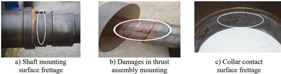
Fig. 2. Thrust collar mountings damages and shaft surface fretage wear
