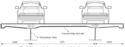
Fig. 5. The standard cross section of single span (Unit: mm)
