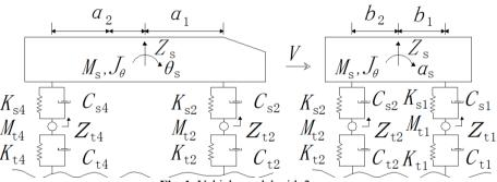
Fig. 1. Vehicle model with 2 axes
