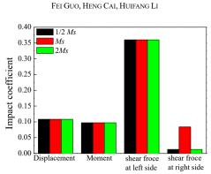
IMPACT COEFFICIENT ANALYSIS ON LONG-SPAN BEAM BRIDGE.
