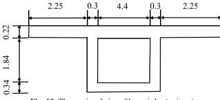
Fig. 10. The sectional size of box girder (unit: m)
