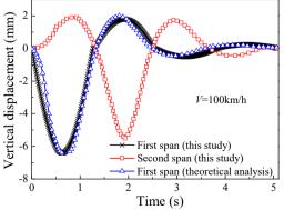
Fig. 6. The displacement responses at mid-span
