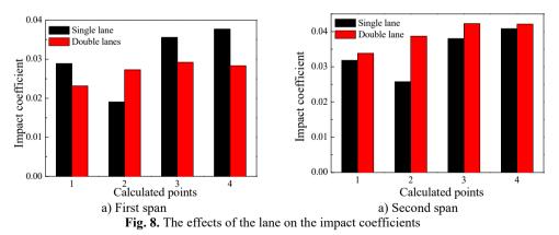
As illustrated in Fig. 8, except for point 2, the global impact coefficient of first span in single lane is greater than that of the double lanes, and it is the same for the local impact coefficient nearby the free end of the cantilever plate. This is mainly attributed the fact that compared with single lane, the lateral load distributions of the bridge deck have changed significantly in double lanes. Whilst for the second span, the global and local impact coefficients of single lane are smaller
