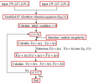
Fig. 4. Calculation process of dynamic response for vehicle-bridge coupling system
