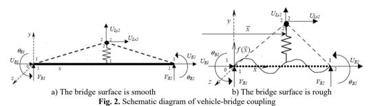
However, the rough bridge surface as shown in Fig. 2(b) will cause the separation between tire and bridge surface, and then contact again, leading to great impact force on the bridge surface. Herein, the random irregularity function  $f(\overline{x})$  is introduced, and the vertical displacement of tire is given by:
