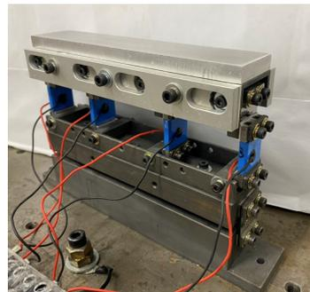
Fig. 6. The picture of the assembled vibratory feeder used in this study
