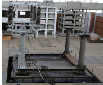
Fig. 5. Site map of Isolating switch vibration reduction test for isolating switch
