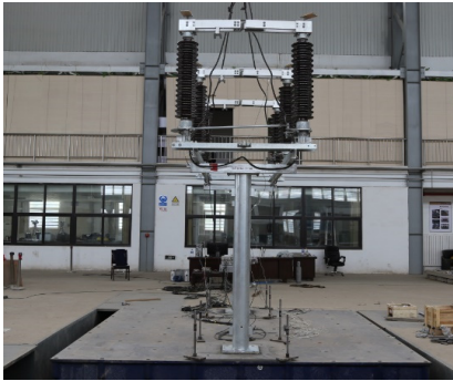
Fig. 4. Site map of seismic test for isolating switch
