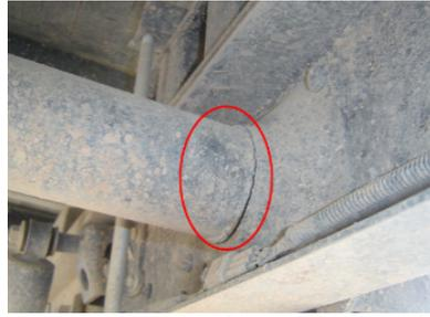
Fig. 14. The weld of the road test result
