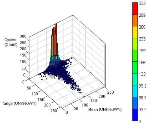
Fig. 9. Rain flow matrix of load spectrum
