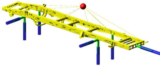
Fig. 5. The frame multi-body model
