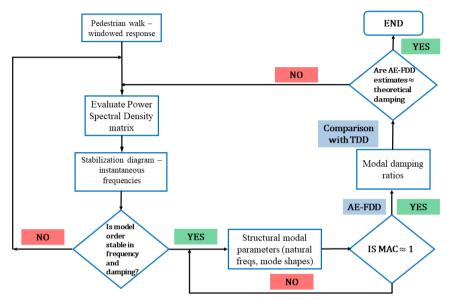
Fig. 2. Methodology of the proposed AE-FDD method for automated damping estimates
