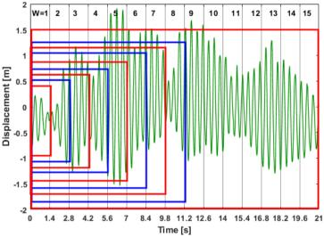
Fig. 5. Vibration response from Daly's bridge automated in 15 windows
