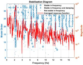
Fig. 6. Stabilization diagram indicating the exact frequencies of the bridge
