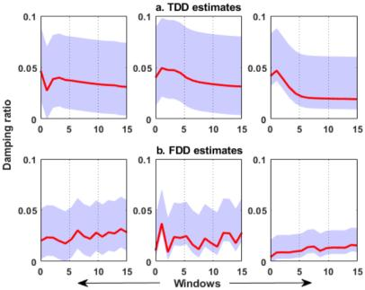
Fig. 8. Evolution of damping ratios for each mode using: a) TDD and b) AE-FDD
