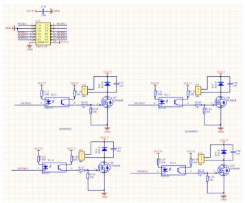
Fig. 4. Fuel injection drives circuit
