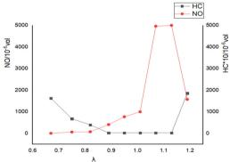
Fig. 6. Engine fuel adjustment characteristic curve
