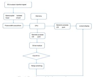
Fig. 1. Experimental device control system
