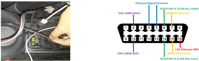
Fig. 3. OBD socket information and pin distribution
