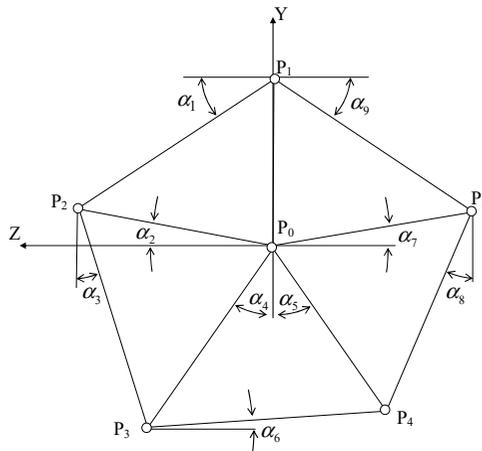
Fig. 3. The scheme of the bore centers in the plane of the carrier cheek  $YZ (P)$  and angular values for trigonometric ratios ( $\alpha$ )
