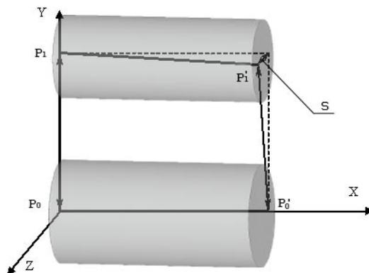
**Fig. 1.** The diagram of measurement of mutual arrangement of bores for axle of the first satellite pinion relative to the central axis of the carrier
