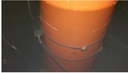
Fig. 5. Symmetrical damage application on the test structure
