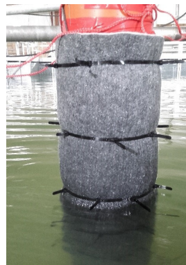
Fig. 4. Synthetic sheet used as marine growth replacement
