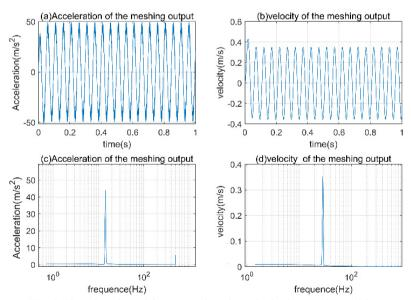
Fig. 6. Time domain and frequency domain under broken tooth conditions
