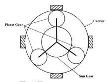
Fig. 1. Planetary gear system
