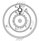
**Fig. 2.** Planetary gear train equivalent mechanical parameters
