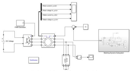
Fig. 8. Completion model for system simulation
