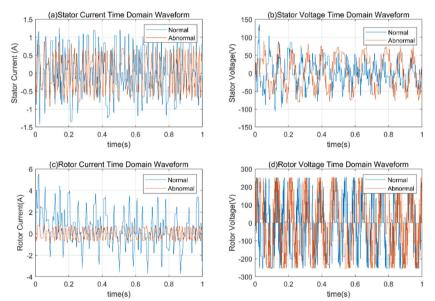
Fig. 9. Generator current and voltage waveform within a second
