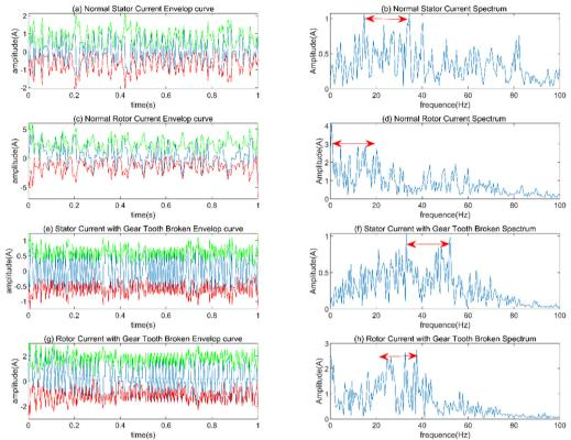
Fig. 11. Envelope curve and spectrum of stator current and rotor current
