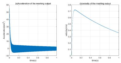
Fig. 5. Acceleration and speed under normal conditions
