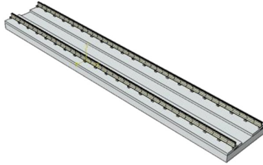
Fig. 5. Finite element track model using ABAQUS software
