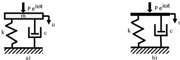
Fig. 4. Calculation model of base with mass  $m$  and without weight
