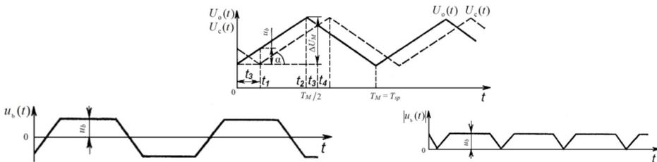
Fig. 3. Time charts of processes inside torquemeter and torsional oscillations measuring device of elastic shaft by differential beat voltage
