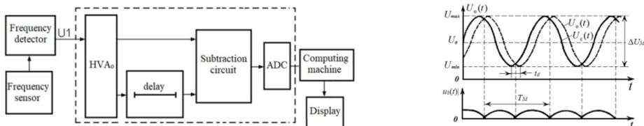
Fig. 5. Measuring calibration circuit, integrated in rotating shafts noncontacting torque meters
