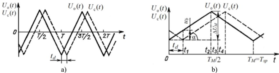
**Fig. 1.** Symmetrical saw-tooth law of: a) HVA high voltage change, b) differential voltage at HVA voltage ramp
