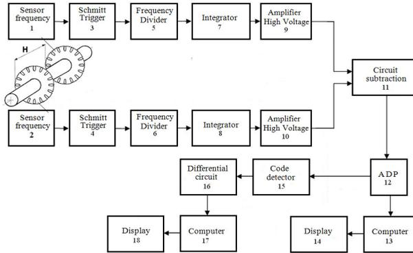
Fig. 2. Structural flow chart of torquemeter and torsional oscillations meter of elastic shaft by differential beat voltage
