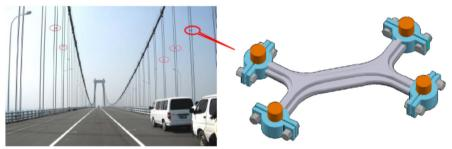
Fig. 1. Sketch of shock absorber
