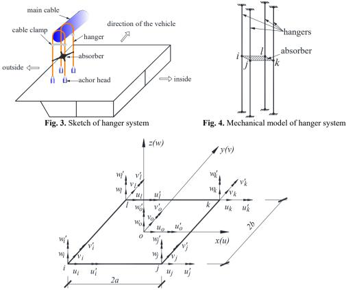
Fig. 5. Nodal displacements of shock absorber element
