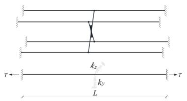
Fig. 6. Hanger system simplified to single cable: a) hanger system with shock absorber, b) single cable with intermediate supports
