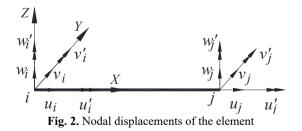
As shown in Fig. 2, the nodal displacement vector of the element is:
