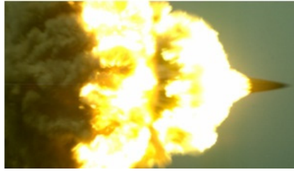
Fig. 6. Photograph of max. area muzzle flame after projectile leaving muzzle brake
