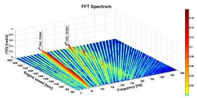
Fig. 5. FFT spectrum of the engine computational model
