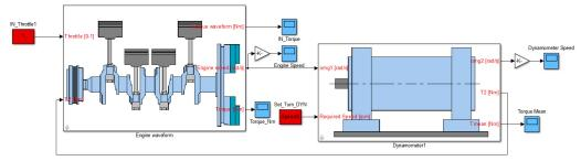
Fig. 3. Computational model of engine and dynamometer
