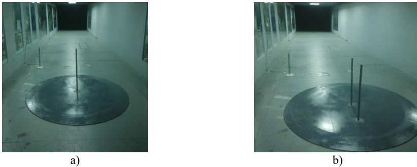
Fig. 2. Installation schematic diagram of wire model in wind tunnel: a) single wire, b) double wire
