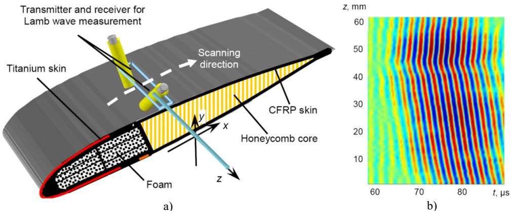
**Fig. 1.** Investigation of the curved surface of the helicopter blade sample using Lamb waves: a) experimental set-up, b) ultrasonic B-scan image of the region between titanium and carbon fibre reinforced plastic (CFRP) skins
