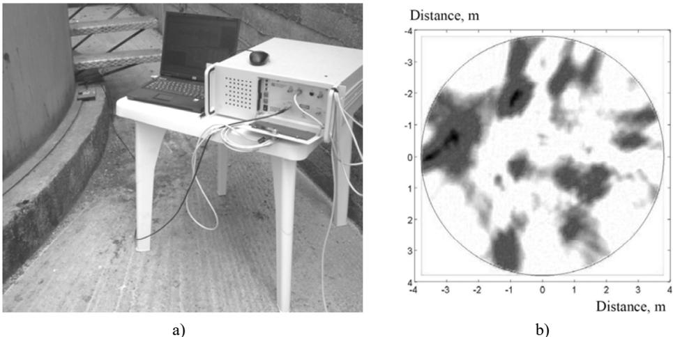
**Fig. 2.** Application of the ultrasonic tomography (transmission) for investigations of real tank floor: a) experimental set-up, b) reconstructed distribution of Lamb waves attenuation inside welded floor of the petroleum tank
