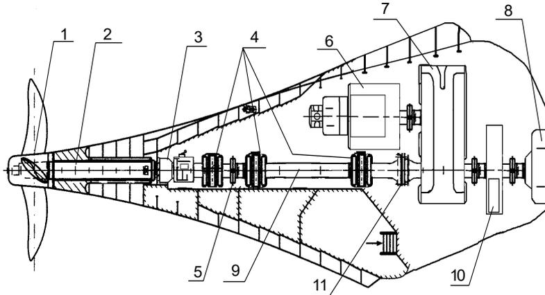
**Fig. 2.** Constructional diagram of the main power plant (MPP) and shafting: 1 – adjustable pitch screw (APC); 2 – the propeller shaft; 3 – mechanism for changing the pitch of the screw SCM; 4 – the basic bearings of sliding; 5 – flange connection; 6 – shaft generator; 7 – reducer; 8 – the main engine (DG); 9 – an intermediate shaft; 10 – a flywheel; 11 – flexible coupling
