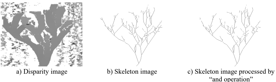
Fig. 4. Disparity image using area-based matching and skeleton image
