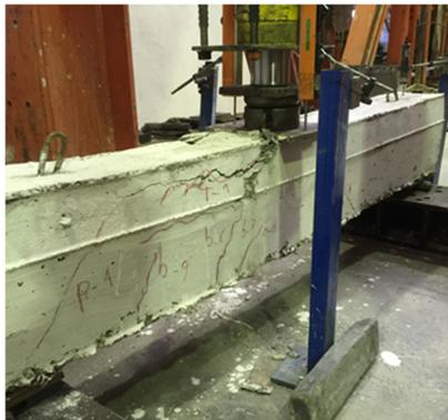
Fig. 8. New model's cracks (ultimate shear capacity)
