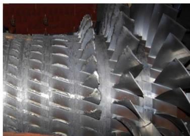
**Fig. 2.** Broken and worn blades
