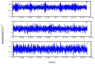
**Fig. 4.** The time domain waveform of the measured fault signal: a) from inner race, b) from outer race, c) from rolling body
