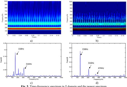
**Fig. 5.** Time-frequency spectrum in *S* domain and the power spectrum of the inner ring fault signal before and after resolution-improvement processing
