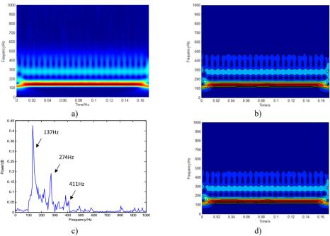
**Fig. 7.** Time-frequency spectrum in *S* domain and the power spectrum of the rolling body fault signal before and after resolution-improvement processing
