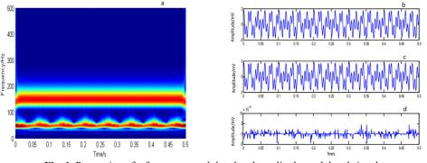
Fig. 1. Procession of a frequency modulated and amplitude modulated signal
