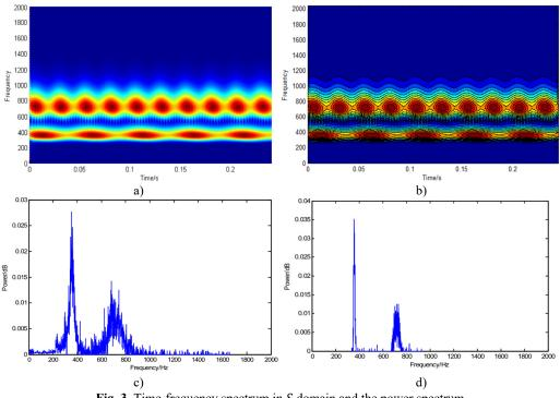
**Fig. 3.** Time-frequency spectrum in *S* domain and the power spectrum of simulated signal before and after resolution-improvement processing
