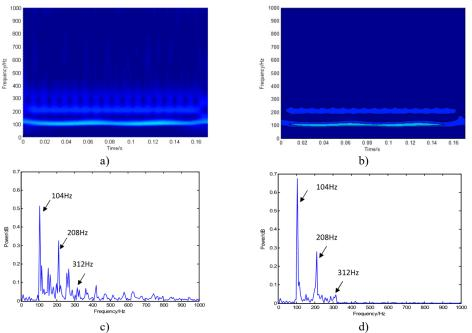
**Fig. 6.** Time-frequency spectrum in *S* domain and the power spectrum of the outer ring fault signal before and after resolution-improvement processing
