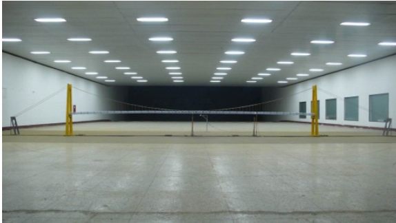
Fig. 9. Full aeroelastic model in wind tunnel
