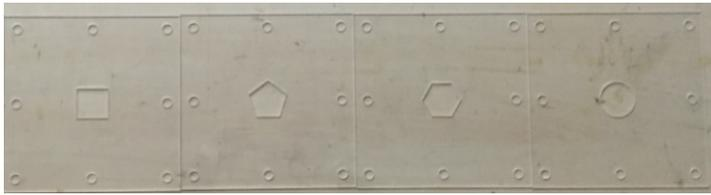
**Fig. 6.** Experimental specimen of various shape orifices
