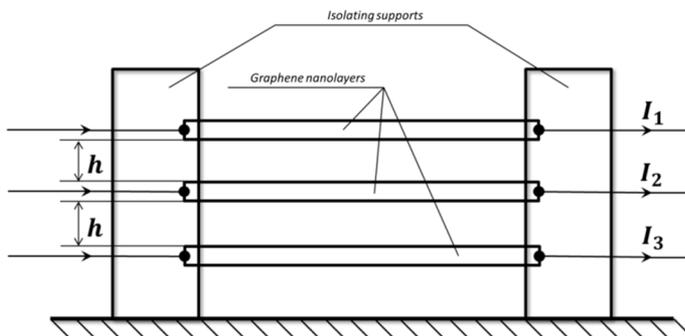
**Fig. 1.** Scheme of a system of nanolayers
