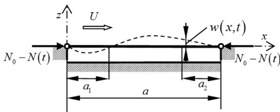
Fig. 1. Stiffened panel in the gas stream
