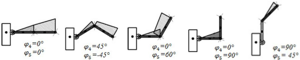
Fig. 2. Diagrams of distribution of forces of resistance along the lengths of the links 4 and 5
