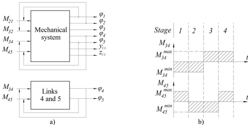
Fig. 3. a) Diagrams of control systems of the mechanical system and links 4 and 5 (horizontal flight and hovering modes), b) cyclogram of control torques of the automatic control system “Links 4 and 5”
