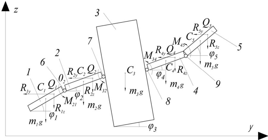
Fig. 1. Analytical model of the oscillatory mechanical system
