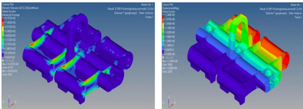
Fig. 1. The largest stress and deformation nephograms
