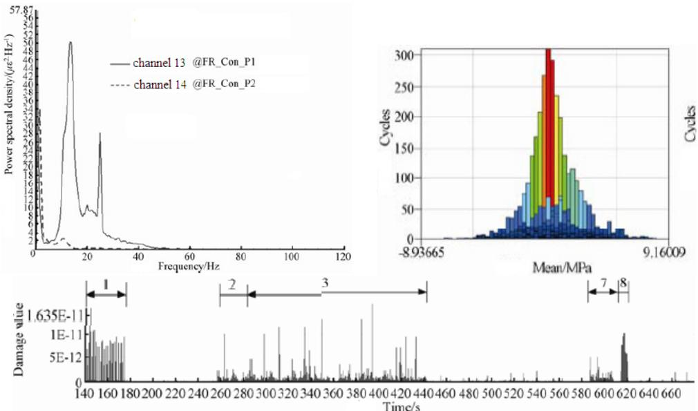
Fig. 2. Fatigue life prediction of the control arm
