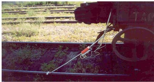
**Fig. 1.** Installation of the sensor of horizontal and vertical movements on the railroad car
