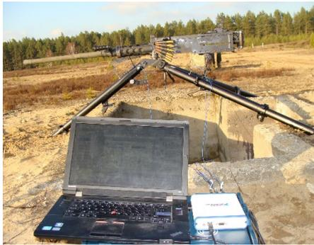
Fig. 4. Recoil force measurement equipment
