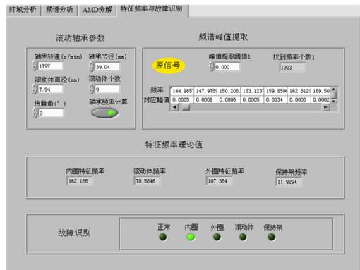
Fig. 6. fault identification module
