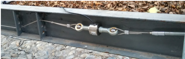
Fig. 2. Anchor device and tension sensor
