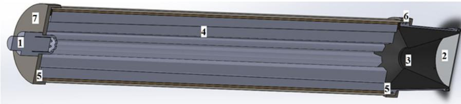
**Fig. 1.** Solid propellant rocket motor components
