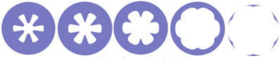
Fig. 2. Propellant grain during burning
