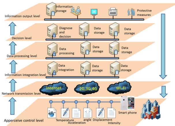
Fig. 1. Framework of cloud-SHM based on smart phone
