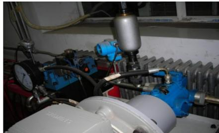
Fig. 2. Plunger pump rig
