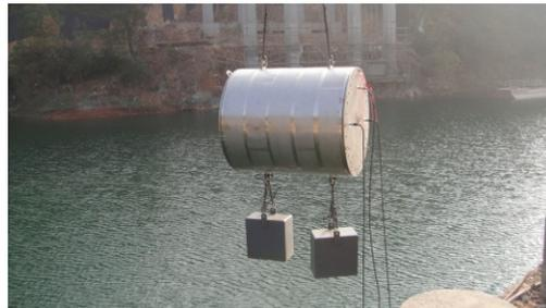
Fig. 1. The double-layer cylindrical shell model
