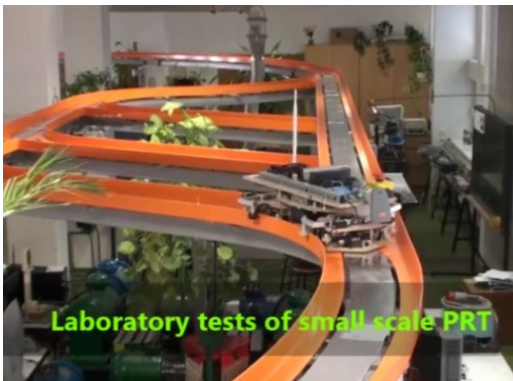
Fig. 1. Experimental track for studies of vehicle dynamics and motion control system operation (Warsaw University of Technology – ECO Mobility)
