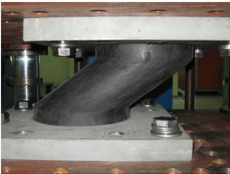
Fig. 3. Specimen under shear loading
