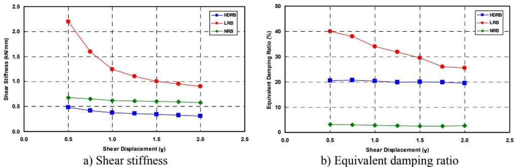
Fig. 8. Effects of shear strain dependency
