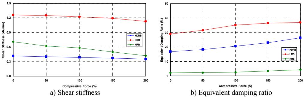
Fig. 7. Effects of compressive stress dependency
