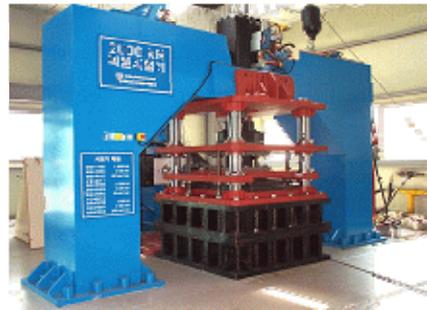
Fig. 2. Compression-shear test machine
