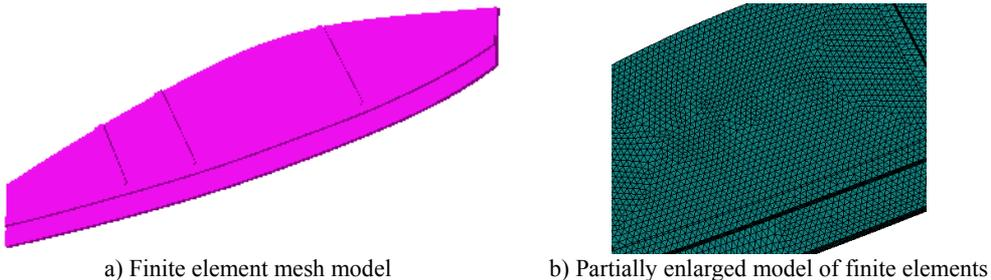
**Fig. 1.** Finite element model of lateral plates
