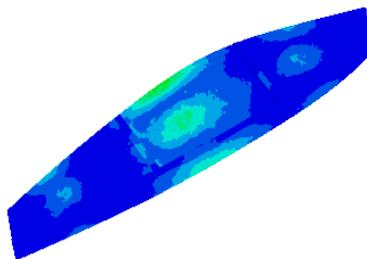
**Fig. 3.** Dynamic stress distribution of lateral plates
