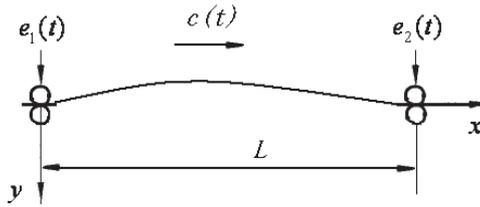
Fig. 2. Axially moving string model with boundary excitations
