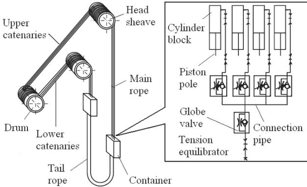
Fig. 1. Schematic diagram of multi-rope friction winder
