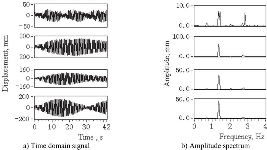
Fig. 4. Time domain and spectrum diagram of lower catenaries transverse vibrations (1# to 4#)
