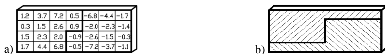
Fig. 1. a) FEM-based optimisation of electrodes topology: cosine values (coefficients of efficiency) ( \times 0.1 ) for two-dimensional piezoceramic element constrained in its central nodes; b) topology of electrodes created referring to personal engineering perception and intuition [4, 5]
