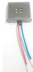
Fig. 11. Horizontal linear vibrating actuator
