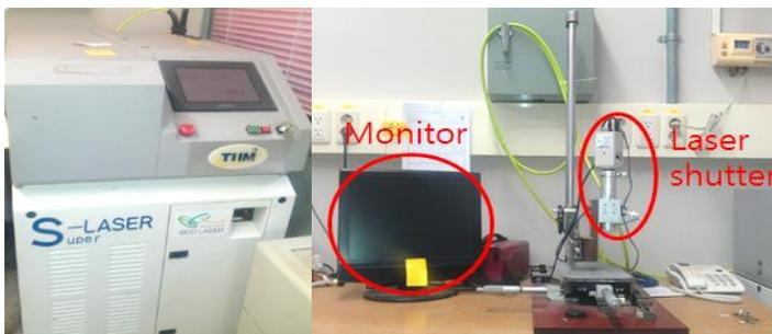
Fig. 10. Laser welding machine set-up
