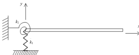
Fig. 3. Spring-dashpot model of cantilever with clearance
