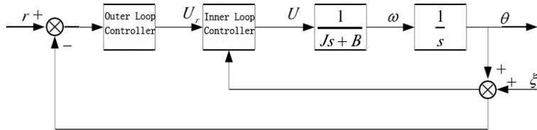
**Figure 10.** Two-ring Control Structure.
