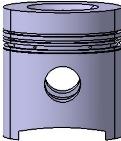
**Figure 1.** Geometrical model for the piston.
