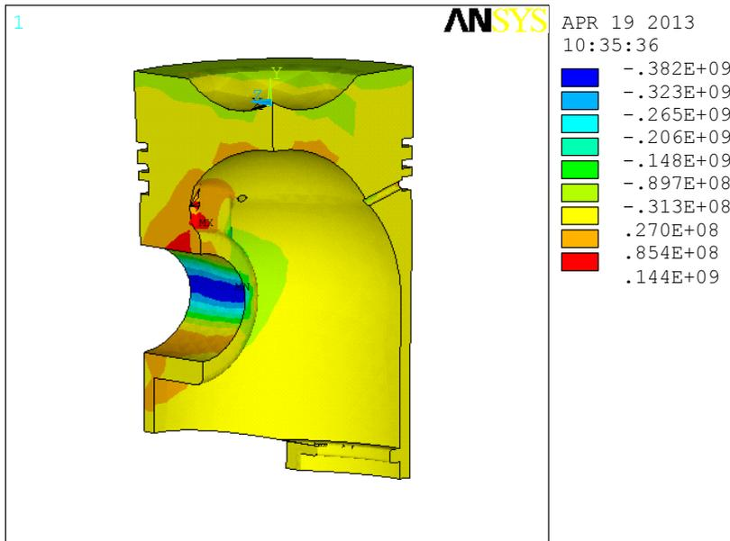
**Figure 3.** Thermo-mechanical coupling stress nephogram.
